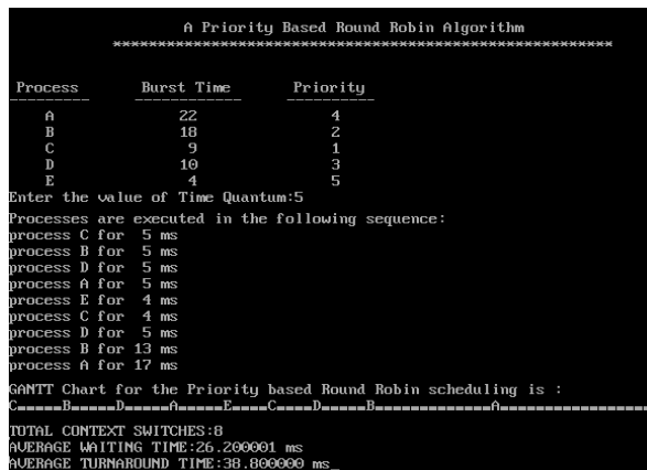
Fig. 2 Priority based round robin for time quantum=5
