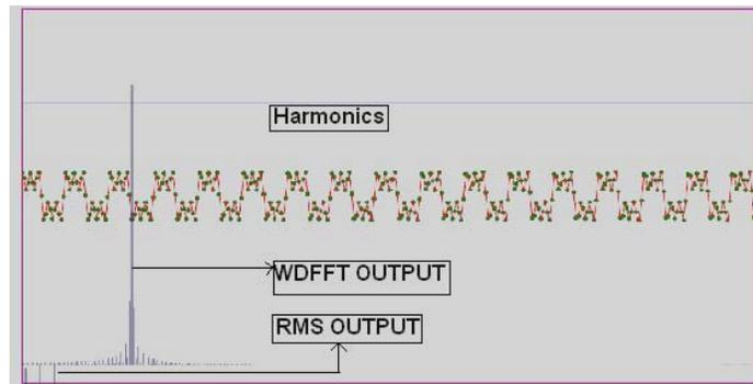
c)  $e(t) = A1 * \sin(\omega t) - A3 * U1*(t-T1)*U2*(t-T2)*\sin(3\omega t) + A5 * \sin(5\omega t) + A7 * \sin(7\omega t)$  (Harmonics)
