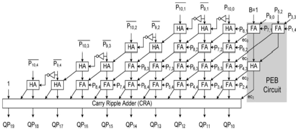
Fig 2. Fixed-width 10 bit multiplier with the proposed PEB circuit
