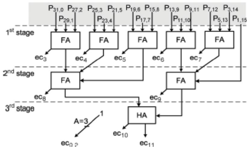
Fig 3. Proposed PEB circuits for L=32 (A=3;B=0)
