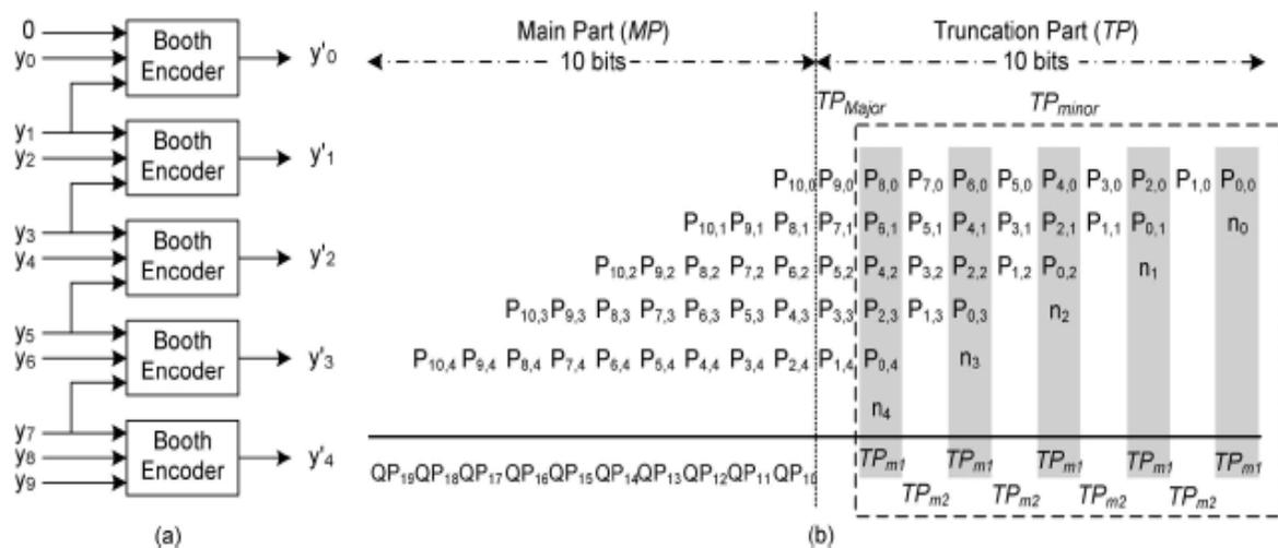
Fig 1. Example of 10 x10 Booth multiplier (a)Booth encoder (b) Partial product array: MP and TP.
