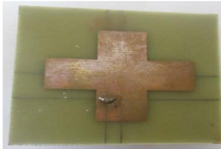
Fig 2(a) Fabricated antenna with top view without EBG structure
