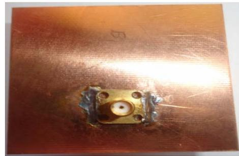
Fig 6(b) Photograph of base antenna with EBG showing bottom view.
