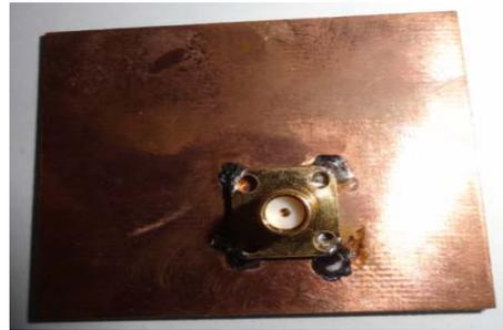
Fig 2 (b) Fabricated antenna with bottom view without EBG structure
