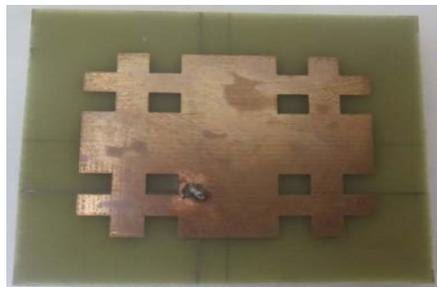
Fig 2(c) Fabricated antenna with first iteration without EBG structure
