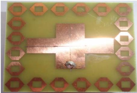
Fig 6(a) Photograph of base antenna with EBG showing top view.
