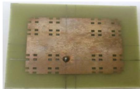
Fig 2 (d) Fabricated antennas with Second Iteration without EBG structure
