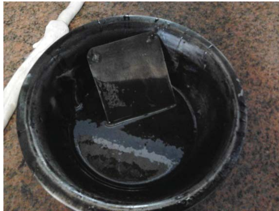
Figure 1. Resin mixed with graphite powder
