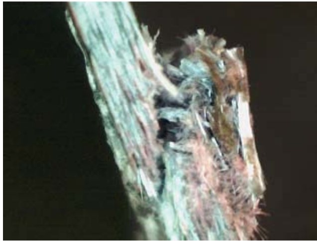
Figure 8. Delamination after CAI test
