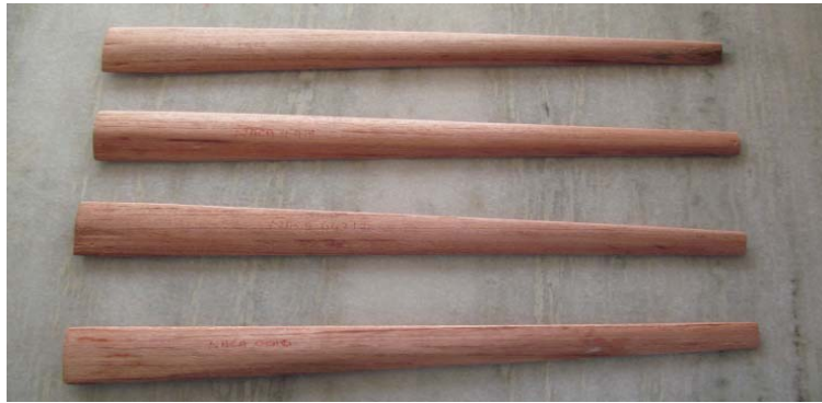
Figure 7. Fabricated NACA 23012,23015,23018,63218 aerofoil profiles blades (F.V)
