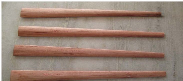
Figure 5. Fabricated NACA 0010,4412,4415,4418 aerofoil profiles blades (F.V)
