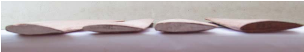
Figure 8. Fabricated NACA 23012,23015,23018,63218 aerofoil profiles blades (S.V)
