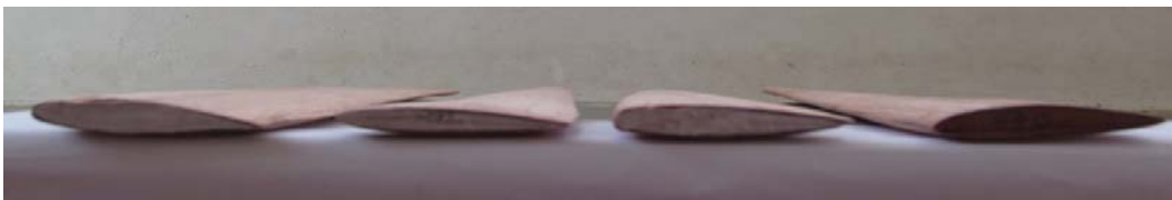
Figure 6. Fabricated NACA 0010,4412,4415,4418 aerofoil profiles blades (S.V)
