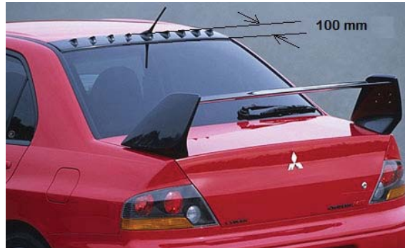
Figure 3. Position of Vortex generators at the rear end of the roof
