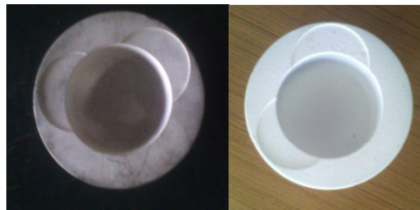
Figure 2: Uncoated piston and Yttrium – Zirconium coated piston
