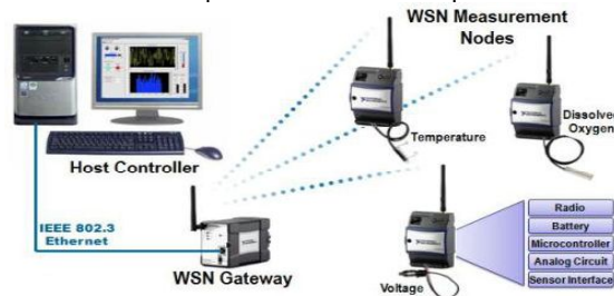
Figure 2: WSN System Architecture
