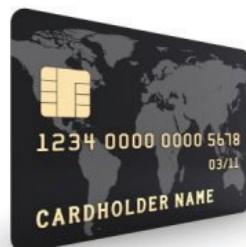
Contact smart cards have a contact area containing a small gold plated contact pad. When inserted into a reader, the contact pad or chip makes contact with electrical connectors that can read data from the chip and write information back. The cards do not contain batteries; the power is supplied by the reader. **Smart card**
