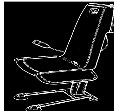
Fig.4. Shows Proposed design of human hoist
