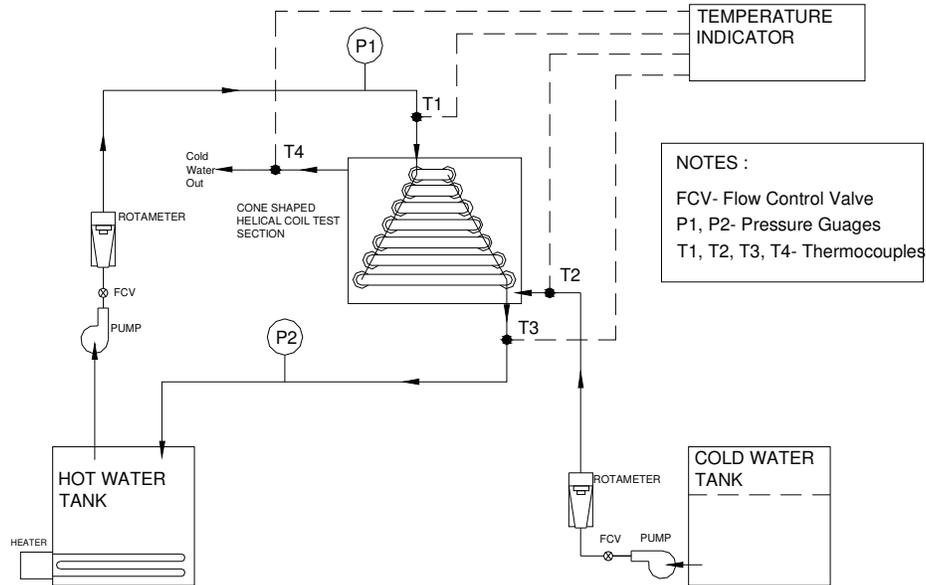
Fig. 1 Experimental set up of cone shaped helical coil heat exchanger
