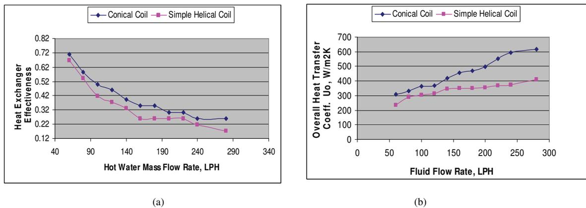
Figure 4.2 (a) Variation of heat exchanger effectiveness with hot water mass flow rate
