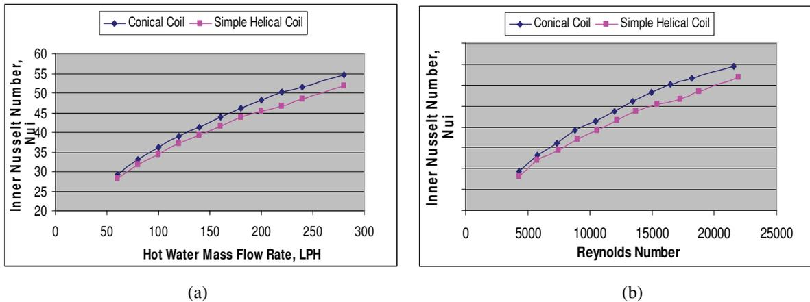
Figure 4.1 (a) Variation of inner Nusselt number with hot water mass flow rate (b) Variation of inner Nusselt number with Reynolds number
