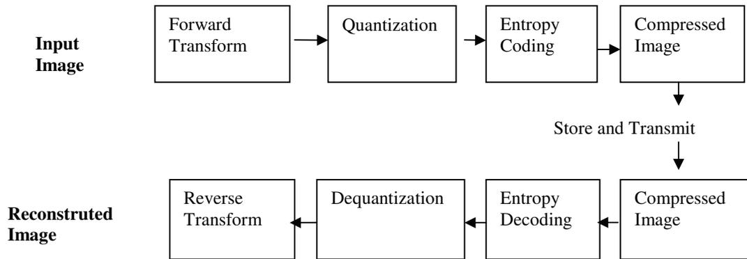
Figure 1. Flow diagram of Image Compression using DWT
