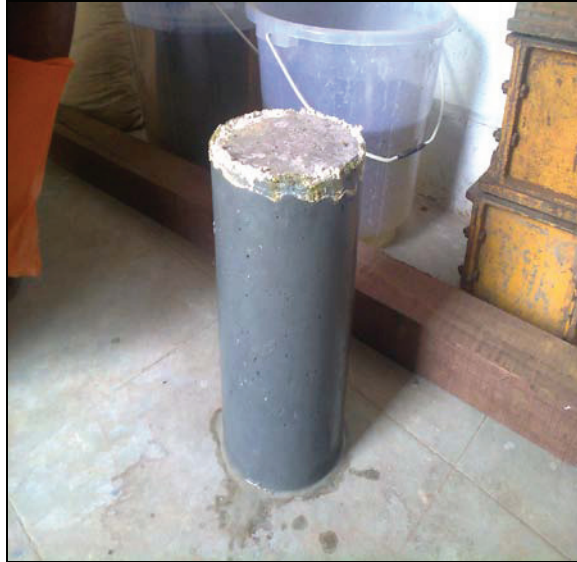
Figure 8: visual appearance heat cured fibre geopolymer concrete specimen after one month of exposure
