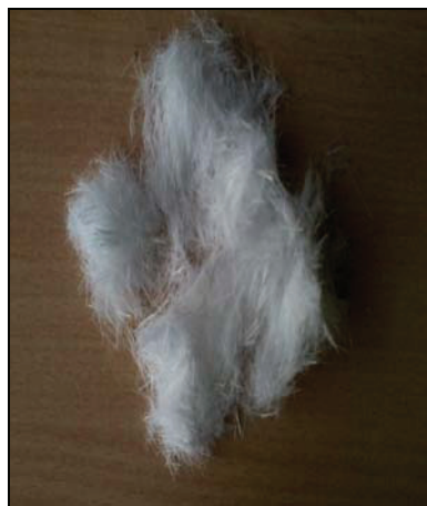
Figure 2: polypropylene fibre (recron 3s)
