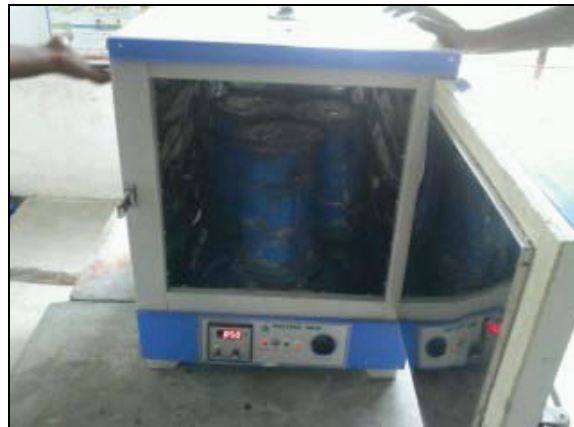
Figure 4: heat curing of fibre geopolymer concrete cylindrical specimen.
