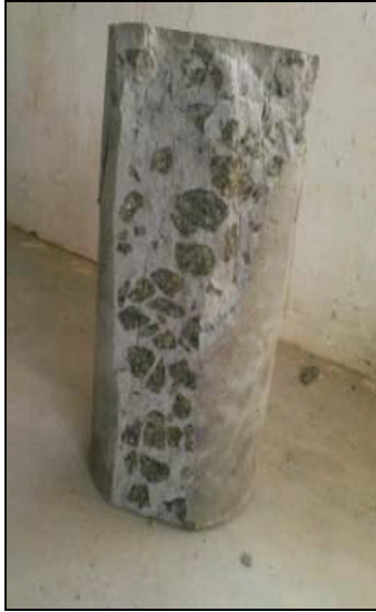
Figure 7: fibre geopolymer concrete specimens after failure
