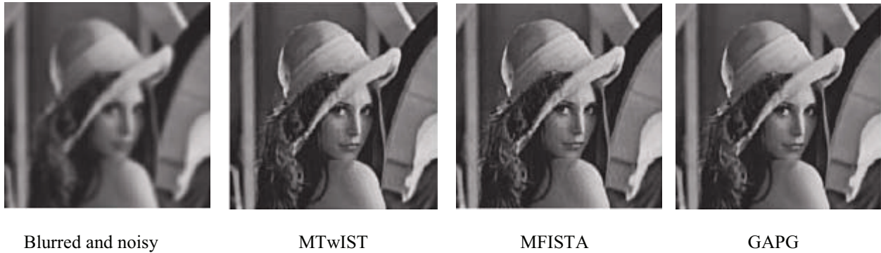
Fig. 1. Isotropic TV-based image restoration from a blurred and noisy Lena image. top left: blurred and noisy Lena; top right: restored image using MTwIST; bottom left: restored image using MFISTA; bottom right: restored image using GAPG.
