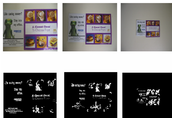
Figure 9 (Row 1) Original indoor images at three different scales (Row 2) Results from edge based algorithm
