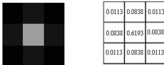
Figure 2 Default filter returned by the fspecial Gaussian function in Matlab. Size [3 3], Sigma 0.5
