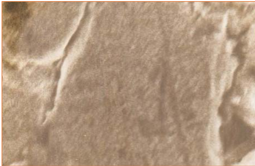
Figure 8: Microstructure showing scale formation on the surface at 1000X
