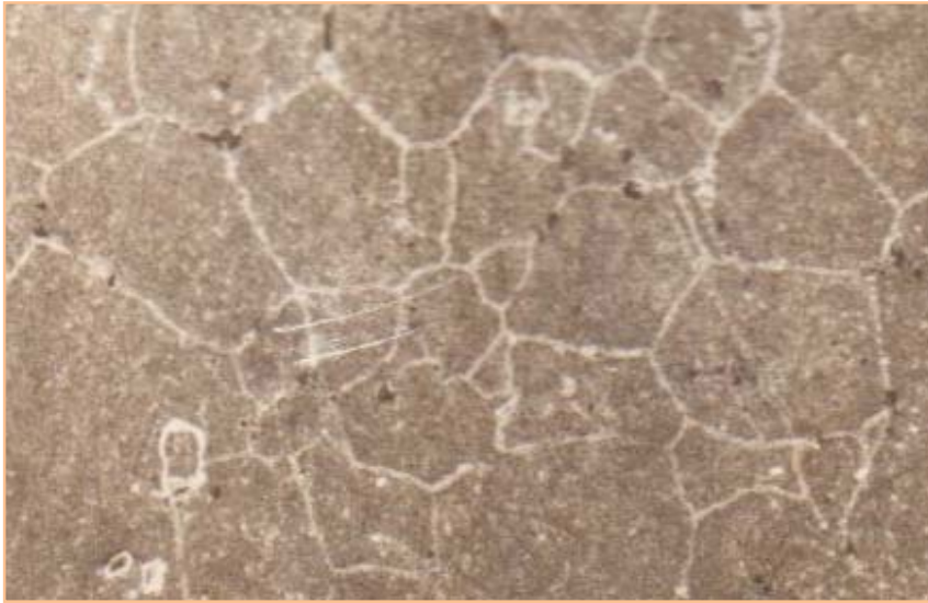
Figure 3: Microstructure of bare sample held at 725°C for 100 Hrs at 350X
