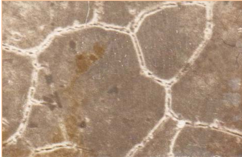
Figure 7: Microstructure of coated sample held at 675°C for 150 Hrs at 500X
