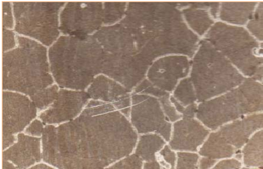
Figure 4: Microstructure of coated sample held at 725°C for 40 Hrs at 350X
