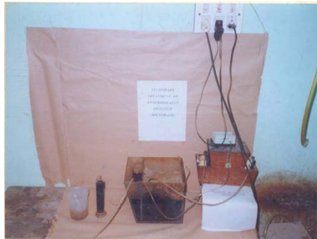
Fig 1. Photograph of Bench Scale Aeration Tank
