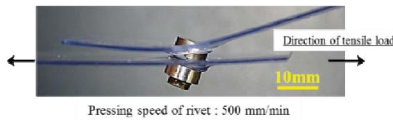
Figure 10. Image of joint fractured by tensile shear test
