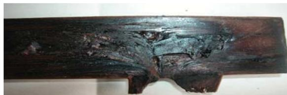
Figure 3. Photograph showing strange expansion on a wood surface occurred during hot-pressing treatment
