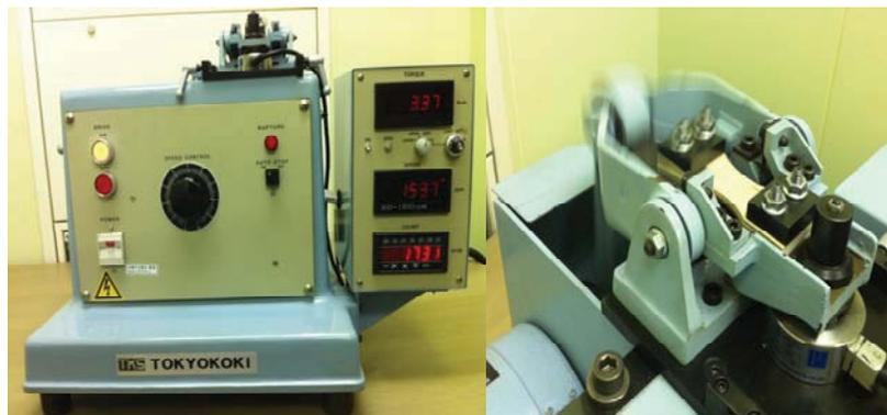
Figure 5. Photograph showing plane bending fatigue testing apparatus
