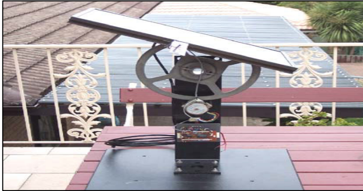
Figure-1: Single-axis rotating PV panel' [2]
