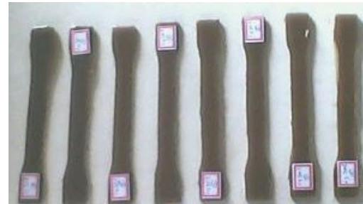
Fig:2.4 Final Specimens for tensile test
