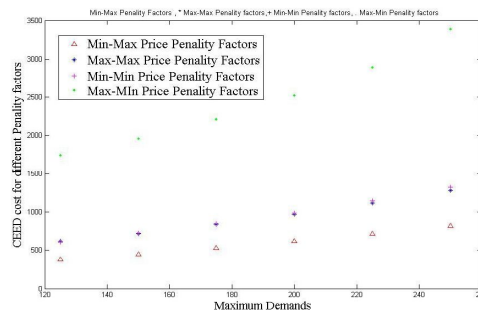
Figure- 1: CEED fuel cost values of the bi-criteria dispatch problem using various price penalty factors
