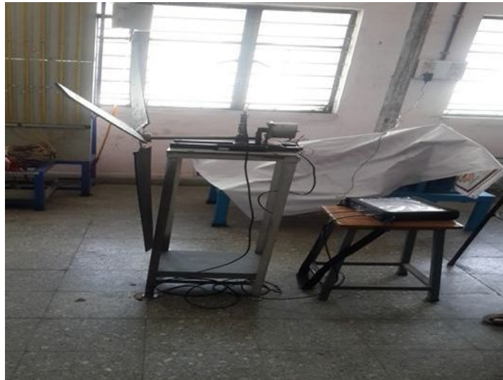
Fig 4.1 Experimental setup of windmill with FFT analyzer
