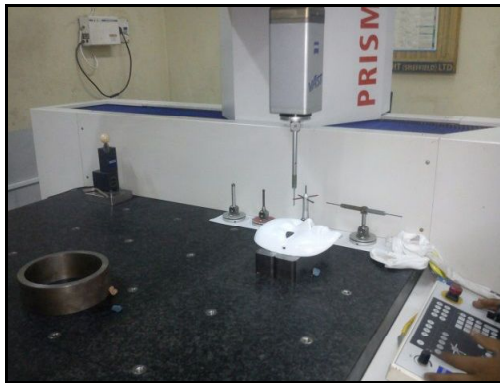
Figure 4 Positioning of mask on CMM
