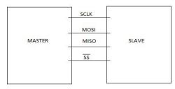
Serial peripheral interface is a synchronous serial data link which operates in full duplex mode. Devices communicate in master slave configuration where the master device initiates the clock and data frame. Multiple slave devices are allowed with individual slave select lines.SPI is a single-master communication protocol. This means that one central device initiates all the communications with the slaves The four basic SPI signals are:
