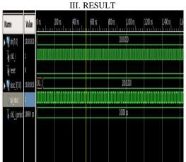
The simulation is verified for the basic SPI read and write operations. The code is also implemented on Spartan 6 FPGA present in UTLP kit.
