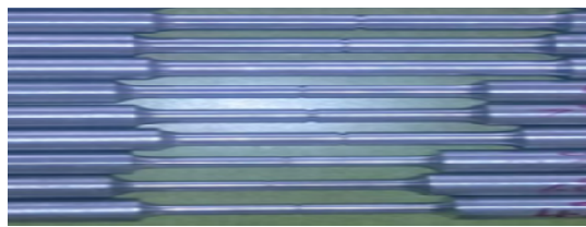
Figure 2. Circumferentially crack round bar testing specimens
