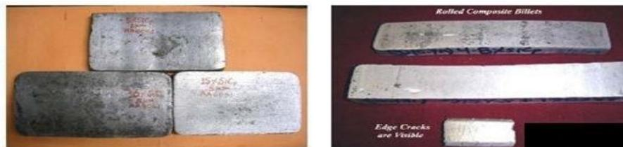
Fig 3: As-cast Composite Rolled Billets
