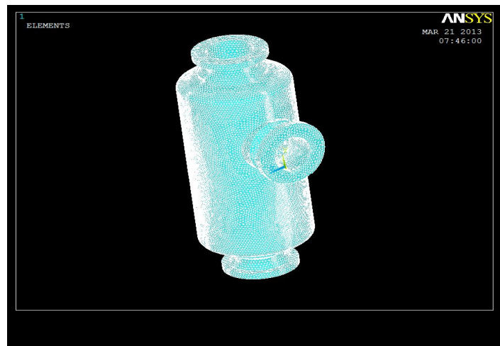
b) Mesh of the pressure vessel
