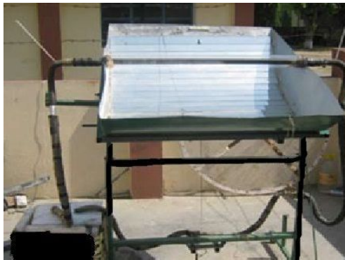
Fig-2 Parabolic trough collector system
