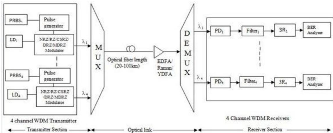
Figure 2. Schematic diagram of WDM optical system using various modulation formats.
