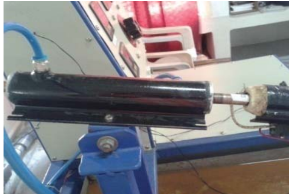
Fig.3 Water Jacket connected to condenser end
