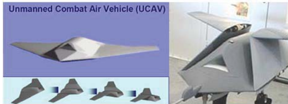
Figure 1. Z-Shaped morphing wing
