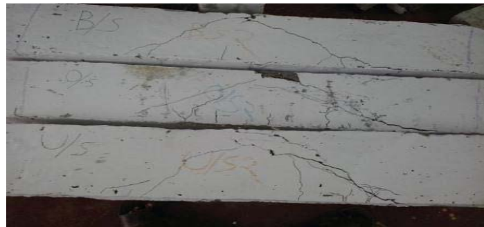
Figure 2. Flexure Failure of over/balanced/under reinforced concrete beam
