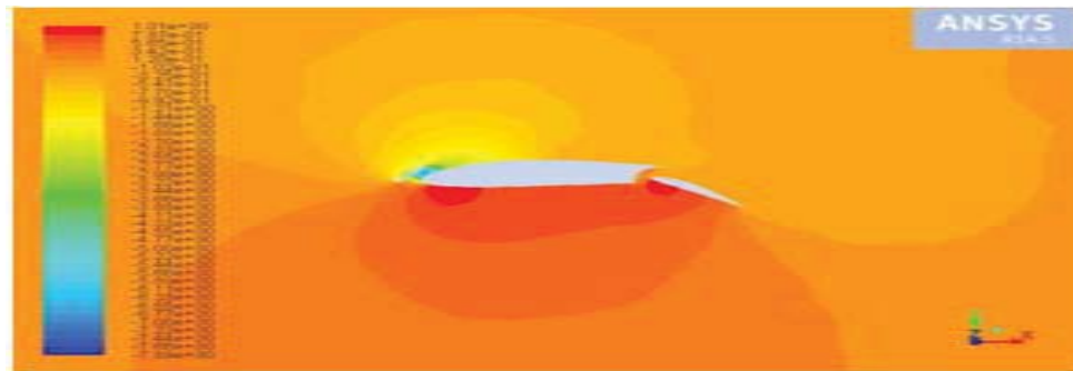
Fig.6. The coefficient of pressure contours on NACA 4415 wing with slat and flap fixed at 30°
