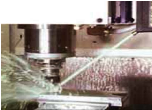
Figure 15. One line coolant flow with high volume of coolant
