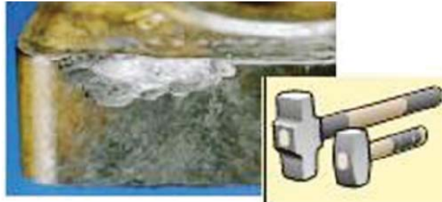
Figure 9. Chipping wear at cutting tool edge [68].
