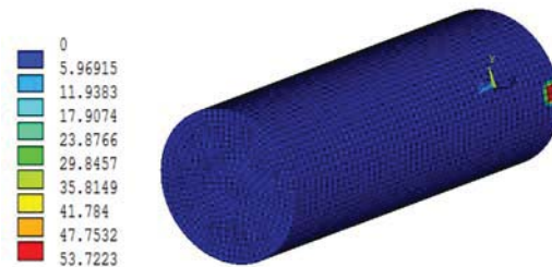
Fig. 1 - Boundary condition and temperature distribution
