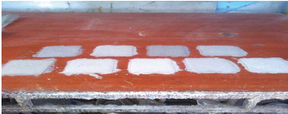
Fig 1: Fabricated of Hybrid GFRP Sheets
