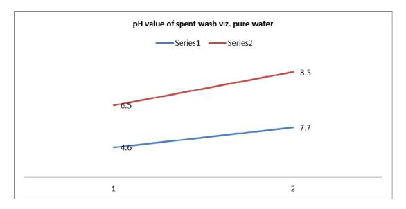
Series 1 is pH value of spent wash before treatment and after treatment Series 2 is pH value of pure water
