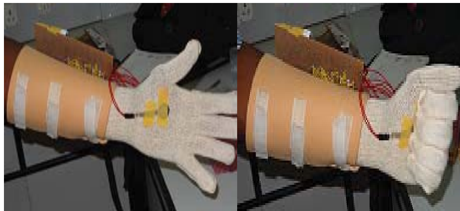
Figure 9: FSR force detection during fist making
