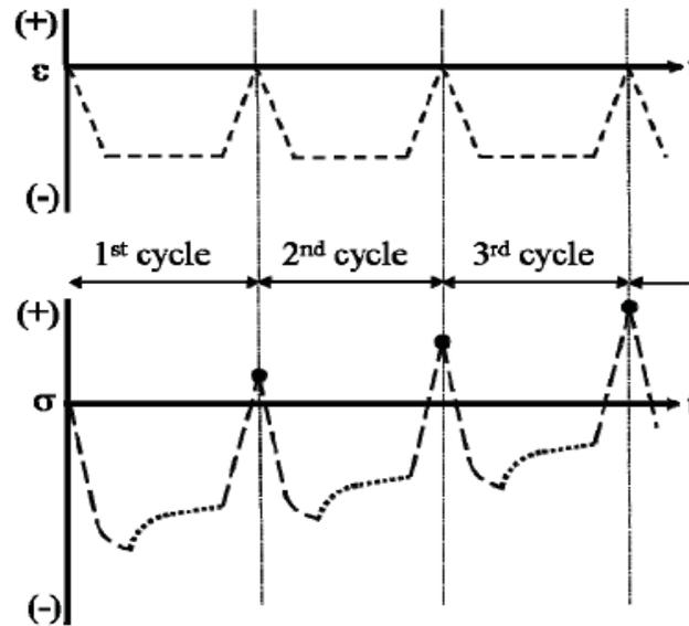
Figure 4. Schematic of applied strain during cyclic loading with compression hold time and the resulting stress response evolution with time
