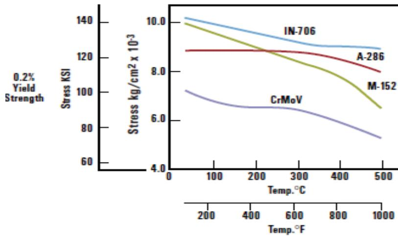
Figure 9. Tensile yield strength comparison
