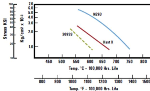
Figure 7 Rupture comparison, N-263Vs Hastelloy- X Vs 309SS
