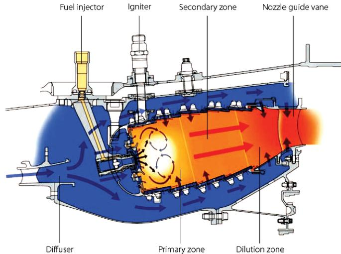
Figure 1. fuel is burned in the combustion chamber at temperatures of over 2000°C, about half the temperature of the sun.
