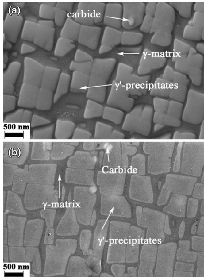
Figure. 5. Microstructure of IN 713 produced by MIM in the “as sintered” state, (b) microstructure of MAR-M247 produced by MIM in the “as sintered” state.
