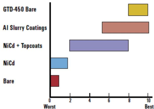
Figure 10. Acidic laboratory tests
