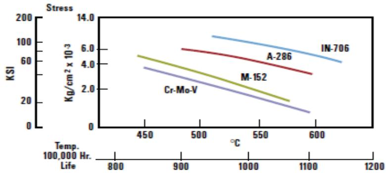
Figure 8. Stress rupture comparison
