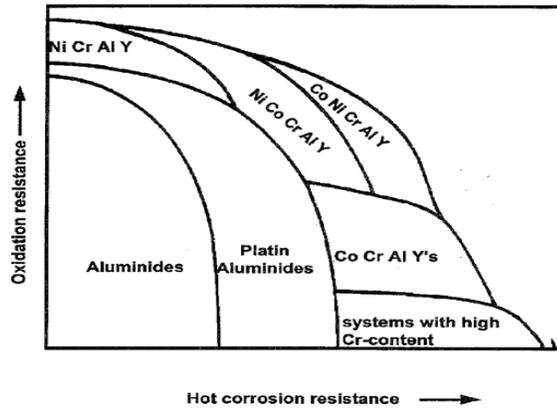
Figure. 3 Oxidation and corrosion resistance of different types of coatings
