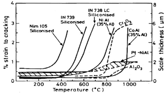
Figure 6. Ductile-to-brittle transition temperatures for diffusion coatings
