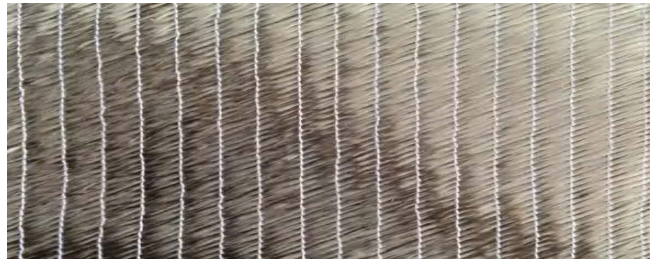
Figure 2. Multi-directional basalt fibre cloth
