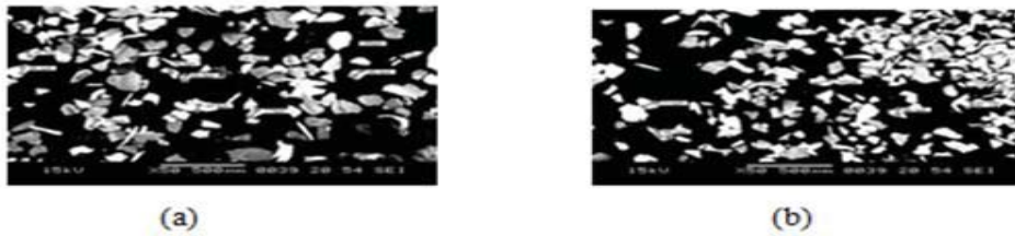
Fig 8 SEM images of debris of coating samples (a) WC sample, (b) Cr3C2 sample
