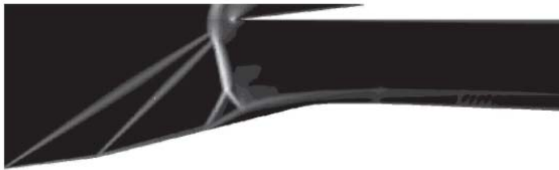
Figure 2. Density gradient contour using k-w turbulence model Flow unstart without cowl bending[10]
