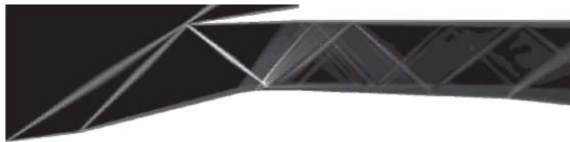
Figure 3. Density gradient contour using k-w turbulence model for q = 2^\circ Flow start with cowl bending[10]
