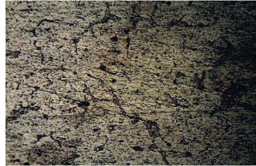
Fig 5: Microscopic Image Of Sample cooled in Oil bath
