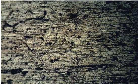
Fig 6: Microscopic Image Of Sample cooled in water bath
