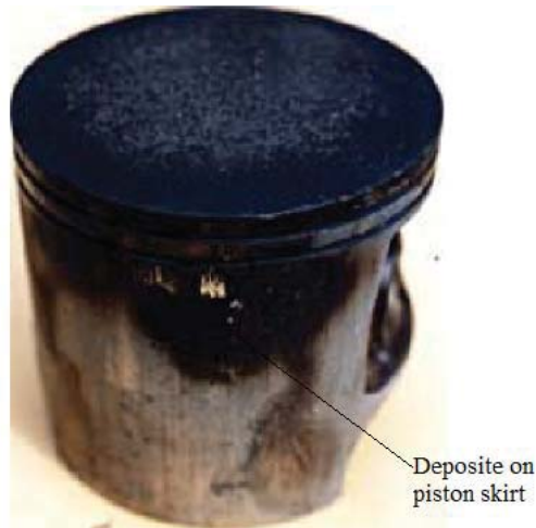
Fig.7 Piston skirt shows deposits
