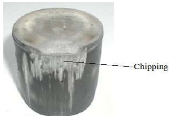
Fig. 4 The piston crown is chipped along the top ring groove.
