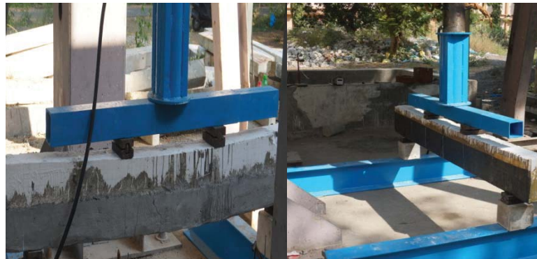
Figure 4. Testing of retrofitted beams
