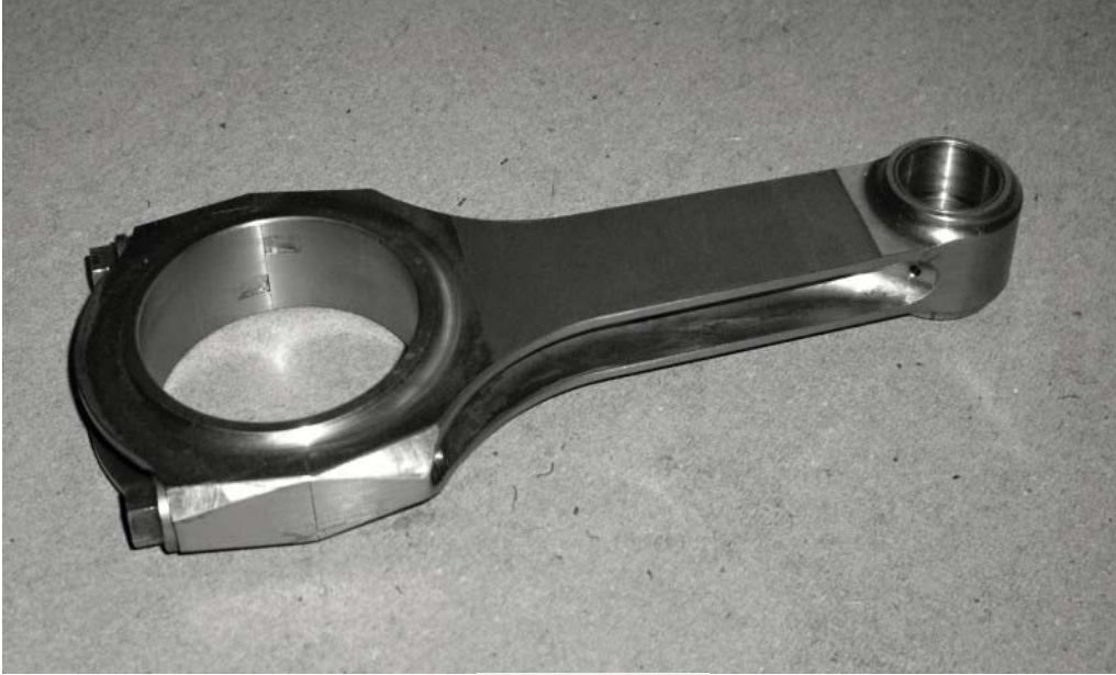
Fig 5. Titanium connecting rod
