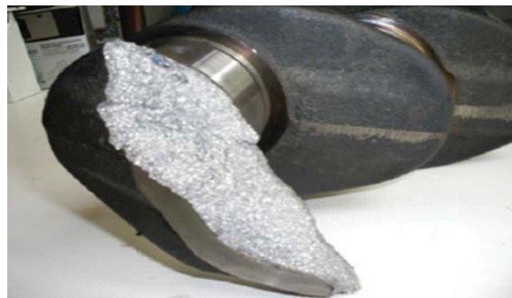
Figure 10. Failed section of crankshaft [3]
