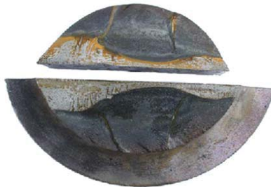
Figure 14. Fracture surface of shaft [4]
