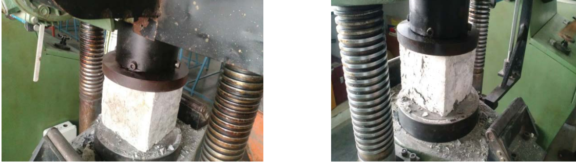
Fig 7 Compressive Strength testing
