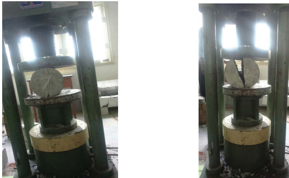
Fig 9 Split Tensile Strength Testing
